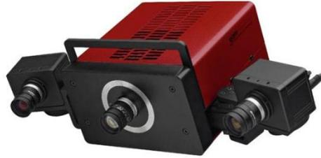
**Fig. 1 GOM ATOS I scanner which was used to digitize the lantern housing.**
