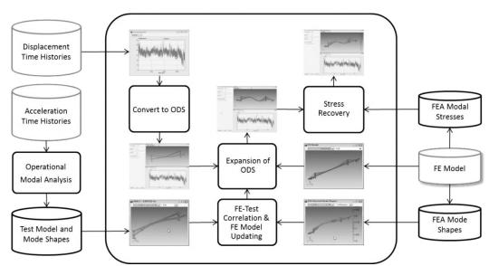
Figure 6 : Processing of the displacement and stress data.
