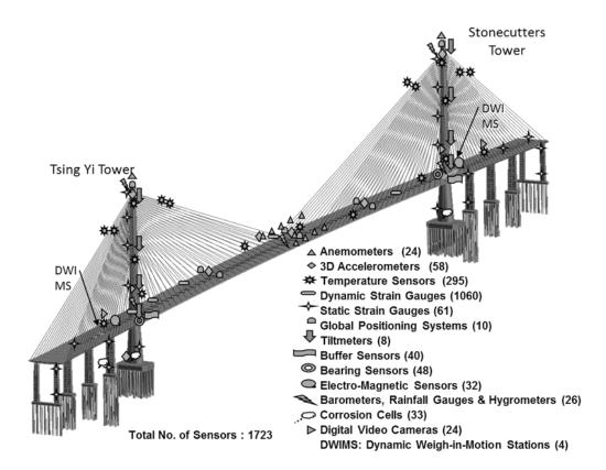
Figure 1 : Layout of sensory systems on Stonecutters Bridge.
