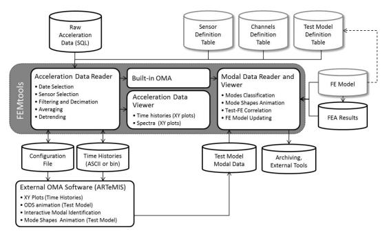
Figure 2 : Processing of acceleration data.
