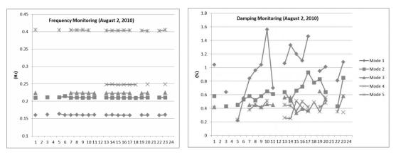
Figure 4 : Frequency and damping tracking during 24 hours.
