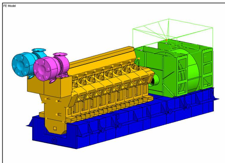
*Fig.7 The Superelement Assembly*
