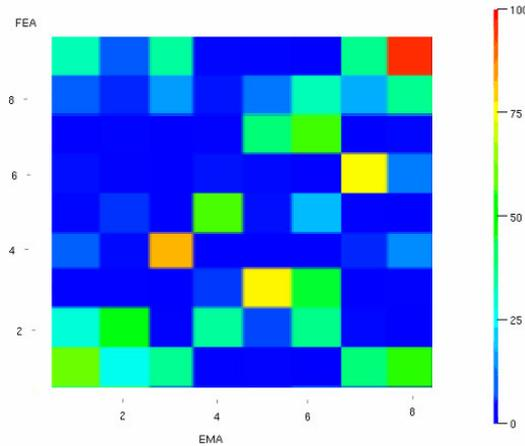
*Fig.4 CROSSMAC matrix Numerical Vs Experimental-rigid body modes*
