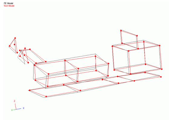
*Fig.10 FEA #6 vs EMA #6 – 16.8 Hz
