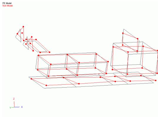
*Fig.9 FEA #7 vs EMA #6 – 16.8 Hz
