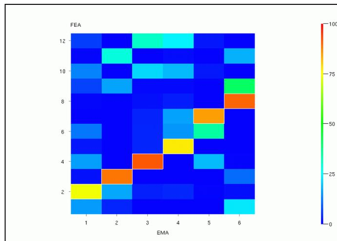
Fig.8 CROSSMAC matrix Numerical Vs Experimental after LOCAL updating
