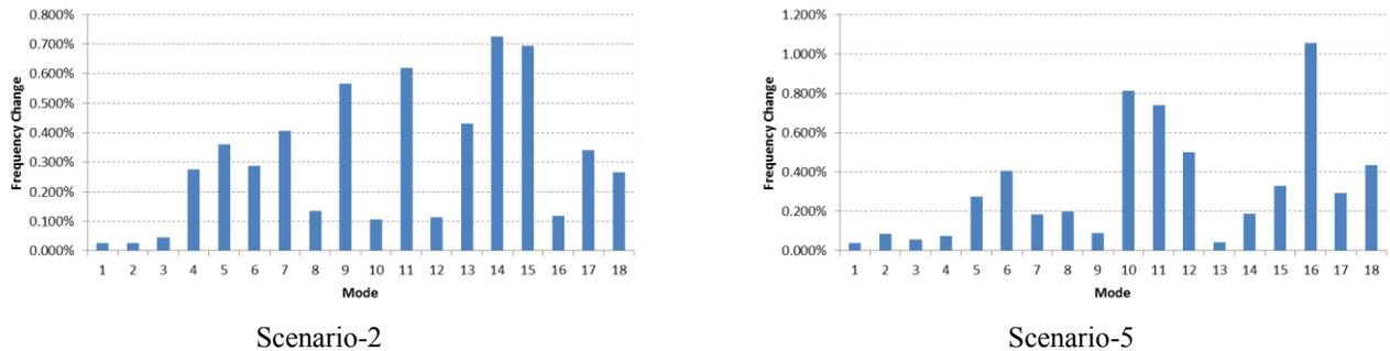
**Fig. 6 The impact of two damage scenarios on the frequencies on the structure.**
