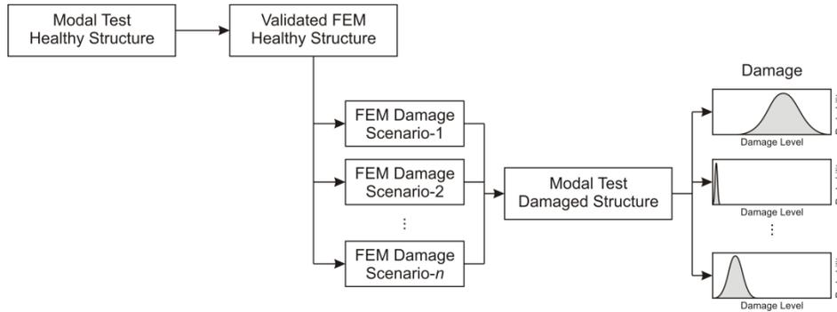
**Fig. 1 The scenario-based damage identification technique.**
