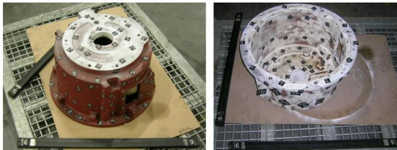
**Fig. 2 The lantern housing during the digitizing process.**
