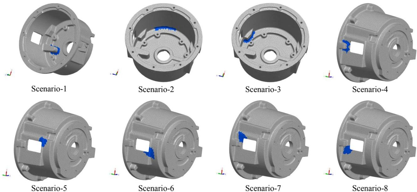
**Fig. 5 Eight damage scenarios (damage area marked in blue).**
