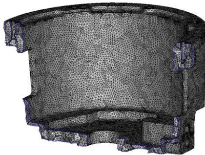
**Fig. 4 Resulting 10-noded tetrahedron mesh**
