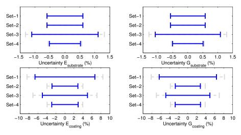
Figure 2: The standard combined uncertainty for the elastic properties identified on the coated steel beams.
