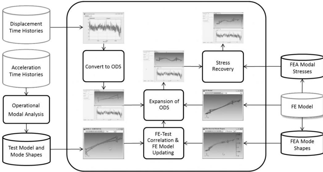
Figure 6 : Processing of the displacement and stress data.
