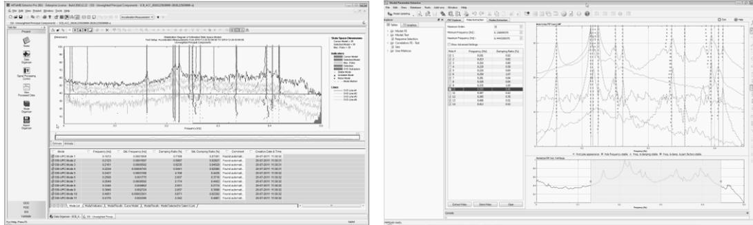
Figure 3 : Stabilization diagrams for SSI (left) and pLSCF (right) methods.
