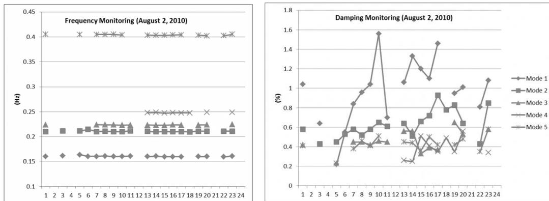
Figure 4 : Frequency and damping tracking during 24 hours.
