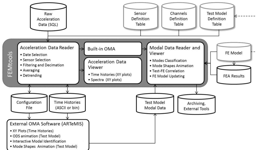
Figure 2 : Processing of acceleration data.
