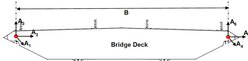
Figure 5 : Layout of the accelerometers on the bridge deck.
