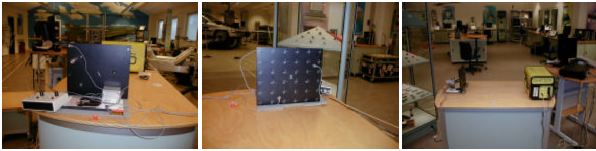
Figure 1: Back, Front, and Side views of test setup showing test object and SLDV
