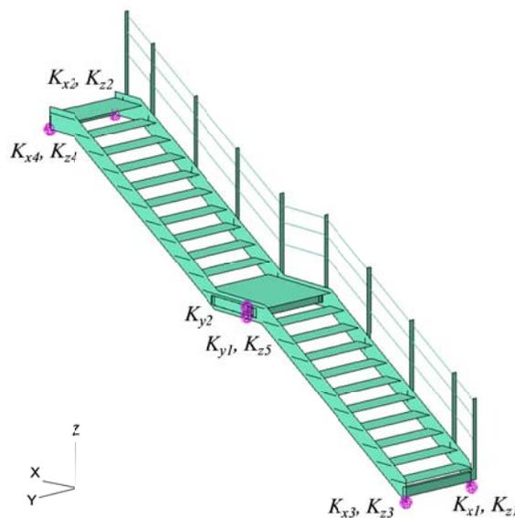
Figure 13. Springs added to the tuned FE model
