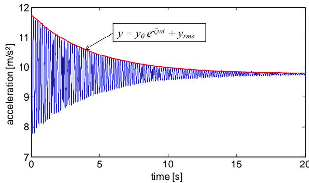
Figure 10. Recorded free decay and free decay response envelope
