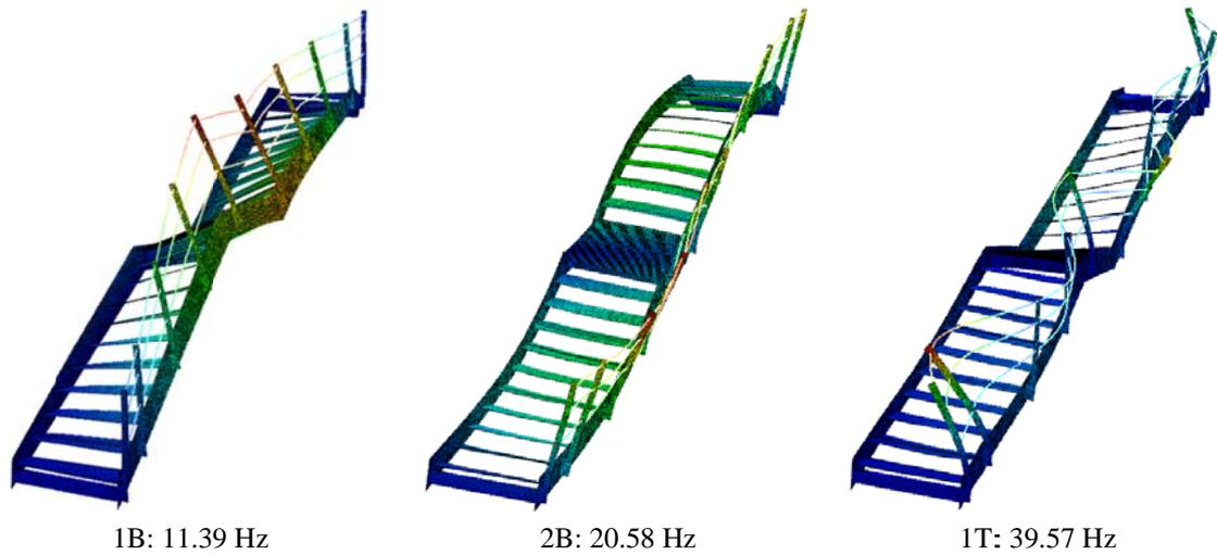
Figure 5. Modes of vibration calculated from the initial FE model
