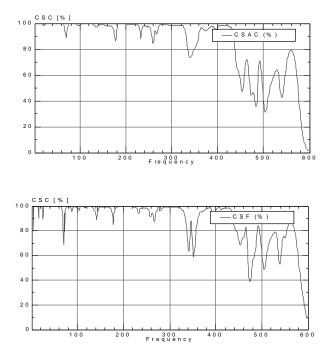
Figure 3. CSAC (top) and CSF (bottom) function after model updating in the 50-250 Hz band.
