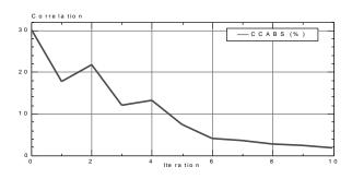
Figure 2. Average residual error of CSAC and CSF as function of iteration loop.
