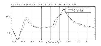
Figure 5. Detail of a test-FEA FRF pair after updating using noisy test data.
