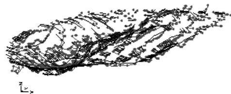
Figure 14: Superposed pair of predicted and measured displacements at excitation frequency 386.2 Hz, showing a FE mesh reduced to the size of the scanning grid.
